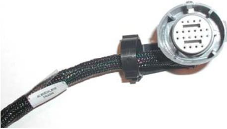
Connect the harness side 20-Pin connector to the stock 20-Pin header connector on the transmission. The location on the transmission where this termination should be made can be seen by clicking on [Twenty Pin Connector Connection](#).
