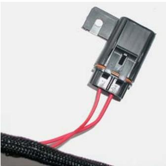
This fuse protects the transmission valve body.
