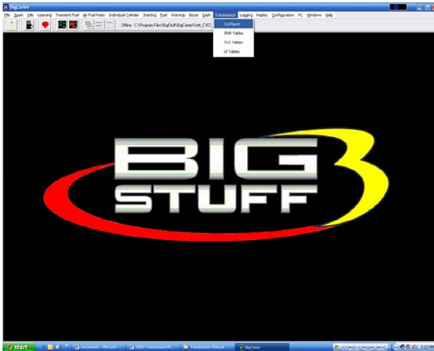
From the main BigComm tool bar, left click on “Transmission”. Keep the left mouse button depressed and slide the mouse pointer down until “Configure” is highlighted.
