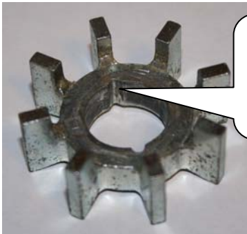
Roll pin slot in-phase with the center of the reluctor.
