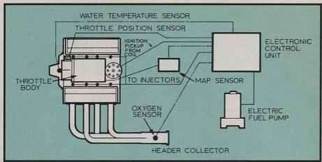
This schematic shows how relatively simple the electronic system is on the DFI injection system. Given eight injectors, there are only six other connections to complete the system. The key to the system is the ECU, which determines the amount of fuel delivered to the injectors based on the engine's fuel needs.
