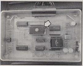
This is an overhead view of DFI's prototype ECU. The rectangular chip (arrow) is the PROM that holds the programming for the fuel delivery curve. Production ECUs will come with three outside diagnostic light-emitting diodes (LED). One light will indicate a TPS failure, one will indicate a MAP sensor failure, and one will indicate that the computer is in the "limp-home mode" (required only if the MAP sensor fails). All the sensors are high-quality GM or Bosch products that are easily replaced.
