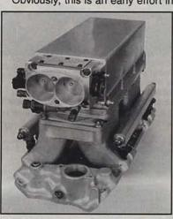
EFI also offers the opportunity to build a slick intake such as this Lingenfelter tunnel ram constructed out of a Weiand Rat motor intake. Note the enlarged throttle body (from a Chevy TPI) and custom fuel rail and injectors at the base of the intake.
