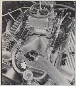
This is the initial prototype system built by DFI that is on its early small-block Camaro. The engine is a Lingenfelter 355 with a Victor, Jr. intake and a 750 Holley carb used as a throttle body with the metering plates and bowls blocked off. Note the fabricated fuel rail and inline fuel pressure regulator (arrow).
