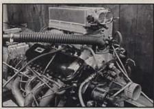
The trick big-block intake was dyno tested on a Lingenfelter 540-cid monster motor against a typical single 4-barrel, single-plane intake, and 850 Holley carburetor. The DFI injection was worth 20 more horsepower at 10-percent less fuel with better idle quality and part-throttle response even with the tunnel ram!
