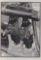
While DFI's early system will not provide for one-off systems, we thought we'd show this photo just to illustrate how easy it is to adapt fuelinjectors to non-EFI intake manifolds. The aluminum adapters are merely epoxied into any manifold and then connected to a custom fuel rail. Simple.
